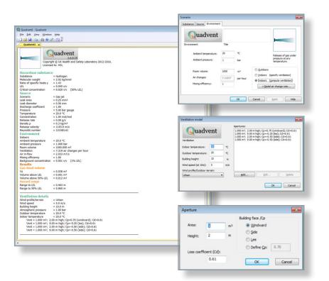
**Figure 2:** Calculation of the hazardous volume,  $V_z$ , using **Quadvent 2** for an indoor hydrogen release at 5 bar gauge. The inset window shows the dialogue boxes for calculating the ventilation rate for a naturally ventilated enclosure.
