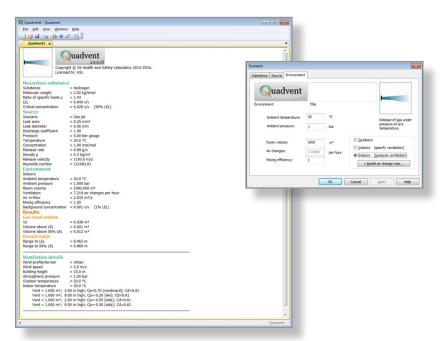
**Figure 3:** Calculation of the hazardous volume,  $V_z$ , using **Quadvent 2** for an indoor hydrogen release at 5 bar gauge. The inset window shows the dialogue box for changing the hole size for a releases under adverse conditions.
