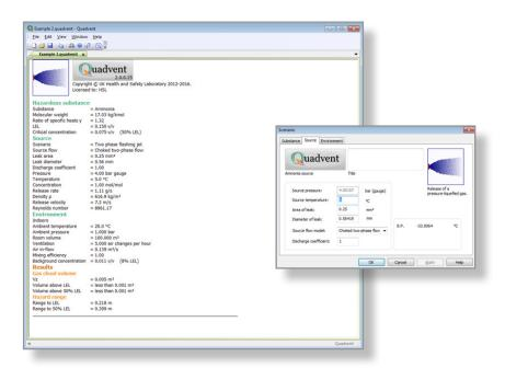
**Figure 1:** Calculation of the hazardous volume,  $V_z$ , from **Quadvent 2** for an indoor release of pressure liquefied ammonia. The inset window shows the dialogue box for inputting or adjusting the details of the source of the release
